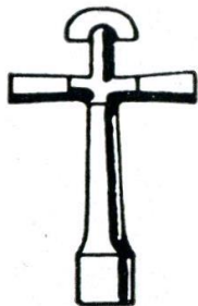
Nr. 131 Kreuzschlüssel aus Messing
