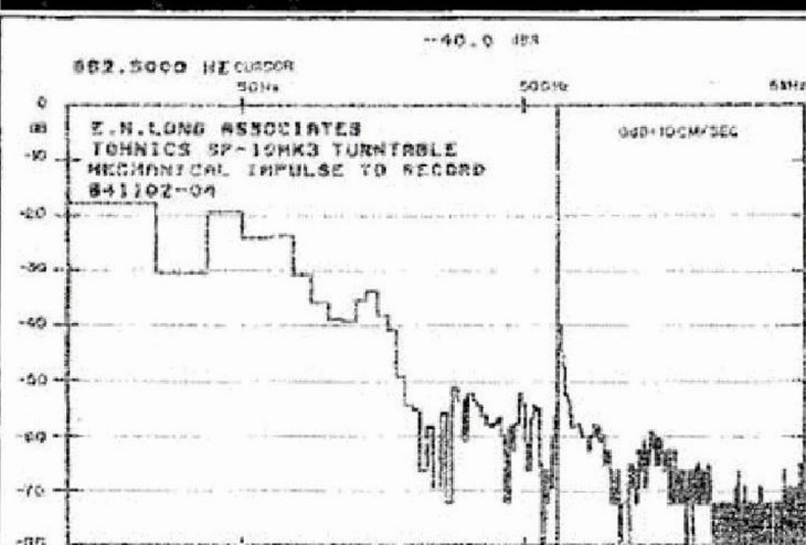
Fig. 5—Spectrum to 5 kHz due to a mechanical impulse applied to the edge of a stationary record with the stylus in a quiet groove. The cursor is at 662.5 Hz, which is the main ringing frequency of the platter and where the output is -40.0 dB below 10 cm/S.
