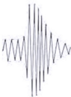
The outline is the envelope, the signal is within the envelope.
