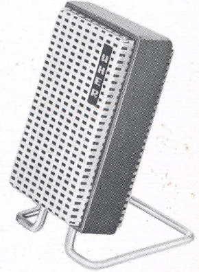
M 531 DYNAMIC MICROPHONE Cardioid response and speech/music switch. Frequency response: 80—12000 cps.
