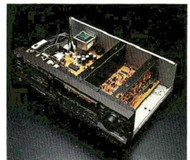
Isolated circuit blocks Blocs de circuit isolés
