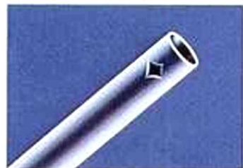
Precision processing of tip mounting hole using a laser beam
