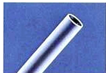
Growing crystals of pure boron into a pipe configuration
