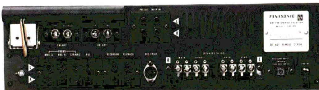
Facilities provided on the rear panel for connection of speakers and numerous Components.
