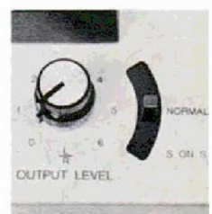
Separate playback controls for both channels. "Sound-on-Sound" switch with 3 positions.
