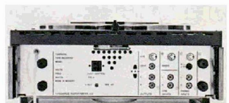
DIN and Phono sockets for connection of radio and record player. There are also a pick-up switch for selection of magnetic or ceramic pick-up, centre channel output, line inputs and line outputs, output for operating voltage for Tandberg FM multiplex filter and socket for remote control of tape recorder.
