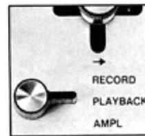
Function selector for each of the 3 main functions of the tape recorder: recording, playback and amplifier.
