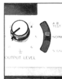
Separate playback controls for both channels. «Sound-on-Sound» switch with 3 positions.
