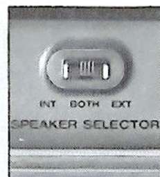
Speaker selector for choice between master, remote loudspeaker, or both.
