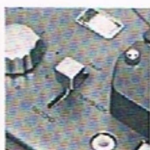
2. Selection of record playback and amplify is accomplished with one knob.
