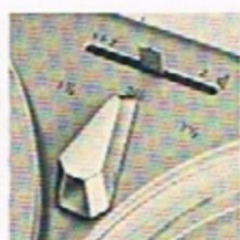
3. Speed selector for 7-1/2, 3-3/4 and 1-7/8 i.p.s. can be operated while the recorder is running.
