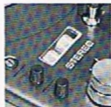
1. The bass can be continuously increased and treble can be continuously decreased by means of individual controls.
