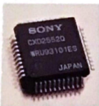
A landmark in digital audio, Sony's CXD-2552 contains the essence of Sony's new High Density Linear Converter™ system.
