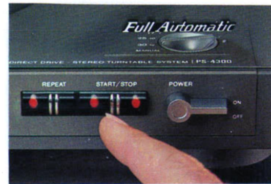
Detail shows touch controls allowing full operation without lifting the dust cover or jarring the unit.
