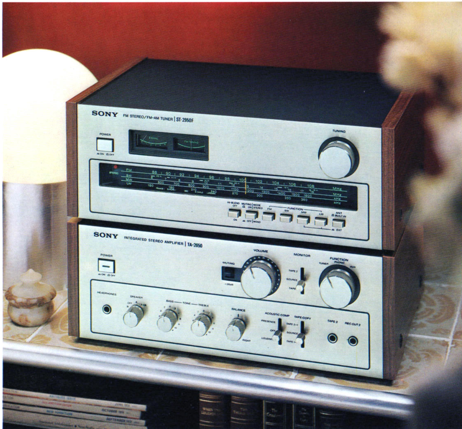
The above detail shows the presence and loudness switch and the second tape input feature on the TA 2650.
