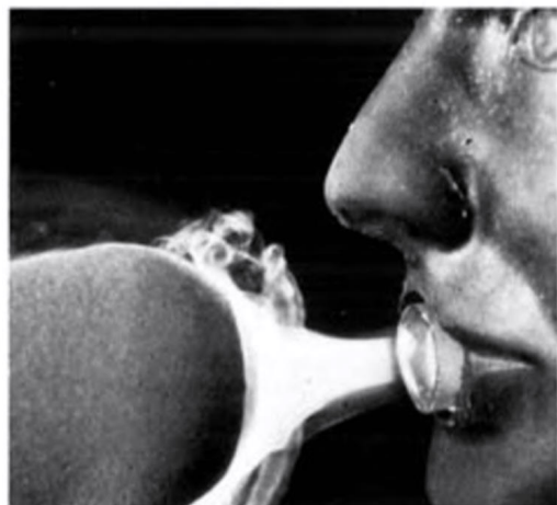
This laboratory test provides a visual representation of the air motion which occurs as a result of breath "pop." It is one of the many application tests used by Shure engineers in determining the optimum size and density of a microphone windscreens.
