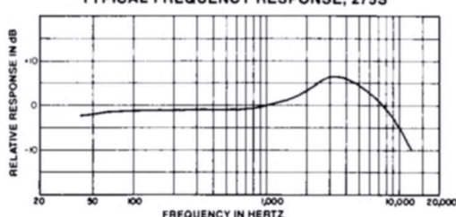
TYPICAL FREQUENCY RESPONSE, 275S
