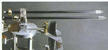
Apply vibrations to the base of a conventional design tonearm; the arm will vibrate together with the base. But the D-O-B tonearm, subjected to the same test, does not vibrate.
