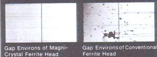
M-C ferrite head resists abrasion much more times than conventional heads. (Enlarged to 500 Times Actual Size)
