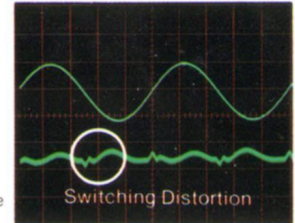
Output Waveform of Conventional Class-B Amp
