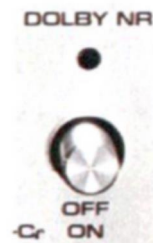
Built in Dolby B noise reduction system on all Pioneer cassette deck (except CT-3131 A).
