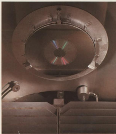
Inspection Player System. Final inspection is carried out with a stereo microscope to confirm surface quality of the CD-Disc Master.
