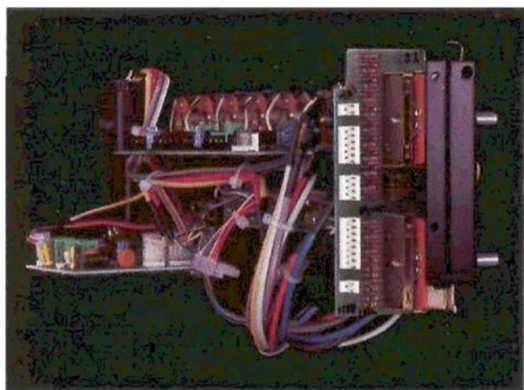
The listen and record selector switches are mounted on the front panel sub chassis. Input selection for each preamplifier originates here by switching dc on these contacts.
