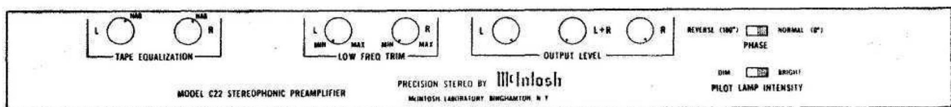
Figure 13. Controls Behind the Front Panel.
