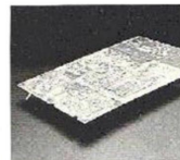
GLASS EPOXY PCB WITH 70 MICRON COPPER
