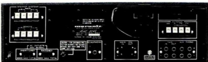
Rear view: Marantz Model 2245 Stereophonic Receiver (90 Watts RMS)
