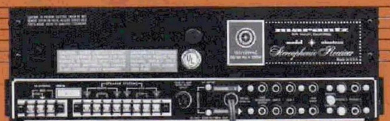
Rear view: Marantz Model 19 Stereophonic Receiver (100 Watts Continuous)
