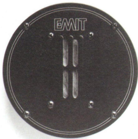
Rotatable Electromagnetic Induction Tweeter. Its etched voice-coil on a planar diaphragm is driven by magnets of rare-earth samarium cobalt, six times stronger than ferrite.
