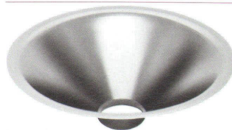
Polypropylene woofer cone. Ideally light, stiff and acoustically inert, it can act as a virtually perfect piston, and without producing internal forms of distortion found in paper cones.
