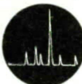
Scanning Function—approximately 250 kHz sweep width—indicates two signals below and three above the received signal, the strongest signal about 30 kHz up the band.
