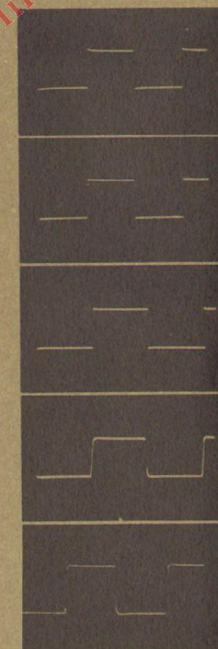
Fig. 5—Square-wave response. Reading from top, 20Hz, 100Hz, 1000Hz, 10,000Hz and 20,000Hz.
