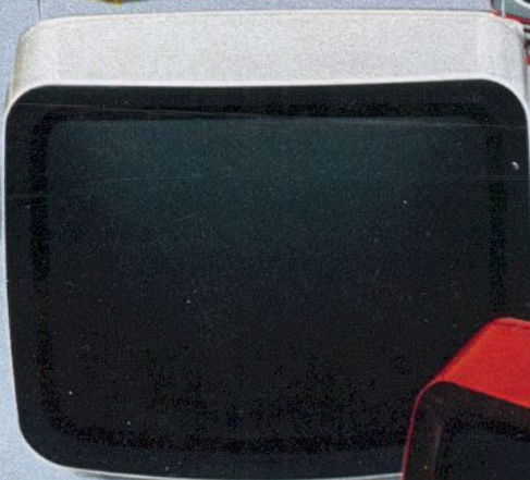
Triumph 2015 Super electronic 51-cm-Bild, Kontrastfilter, 7 Programm-Impulsfelder
