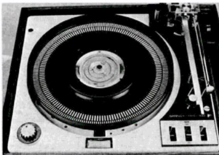
Fig. 3 —With the platter removed and inverted, the two bands of stroboscope lines are seen on the underside of the platter. They are illuminated by a neon bulb and viewed through a mirror visible through the opening directly in front of the platter.
