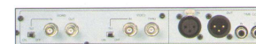
MODEL 8335 TIMECODE/SYNC BOARD This board allows the tape to playback LTC and assemble record externally generated timecode 7-1 TIME can also be converted to LTC. Option of referencing externally to Word, Video or AES/EBU
