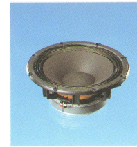
12W-360 12" Woofer PA-D-M* fs: 45Hz Qts: 0.15 Vas: 103.7 SPL: 100dB (1W/1m) Pwr.,rms: 360W Pwr.,mus: 600W
