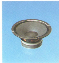
10W-150 10" Woofer PA* fs: 40Hz Qts: 0.26 Vas: 130.5 SPL: 97dB (1W/1m) Pwr.,rms: 100W Pwr.,mus: 200W
