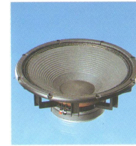
15W-300 15" Woofer PA-D* fs: 31Hz Qts: 0.26 Vas: 262.0 SPL: 99dB (1W/1m) Pwr.,rms: 200W Pwr.,mus: 400W
