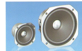
F-120A Fullrange Speaker M-Hifi* fs: 65Hz Qts: 0.50 Vas: 9.0 SPL: 89dB (1W/1m) Pwr.,rms: 30W Pwr.,mus: 60W weight: 2000g
