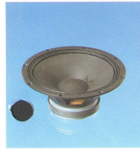
12W-150 12" Woofer PA* fs: 60Hz Qts: 0.41 Vas: 74.0 SPL: 98dB (1W/1m) Pwr.,rms: 150W Pwr.,mus: 250W
