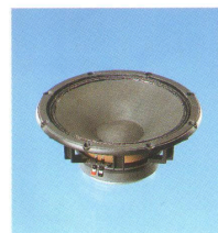
12W-200 12" Woofer PA-D* fs: 60Hz Qts: 0.37 Vas: 76.7 SPL: 99dB (1W/1m) Pwr.,rms: 150W Pwr.,mus: 300W
