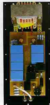
Frequency cross over SN/SL 300
