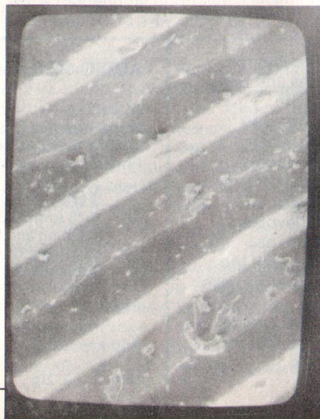
Fig. 1 — Photos through an electron microscope at 500 times magnification showing a new, unplayed disc (left) and one that has been cleaned with Disco Film.
