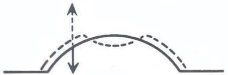
Action of diaphragm at higher frequencies. Dotted line shows departure from piston action.
