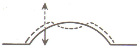
Action of diaphragm at higher frequencies. Dotted line shows departure from piston action.
