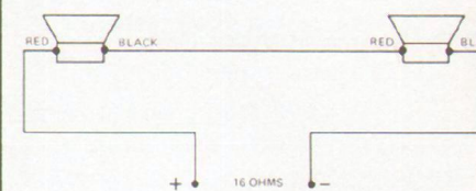
FIGURE 12 Connection of 2 EVM .15L Speakers in Series
