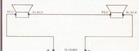
FIGURE 12 Connection of 2 EVM-12S Speakers in Series
