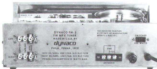
Fig. 1—Rear panel layout of the Dynaco FM-5
