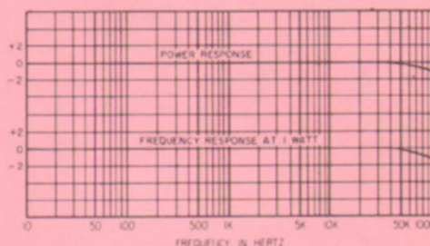
Crown DC300A: Power/frequency response. Power response indicated. 0 dB=200W per channel into 8 ohms.
