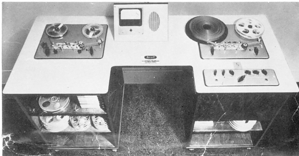
Left — the simple yet ultra-reliable unit produced for continuous music applications. Below is the editing console for producing special tapes for The British Library of Tape Recordings for Hospital Patients. These are made on 16mm tapes at a speed of 2 inches per second
