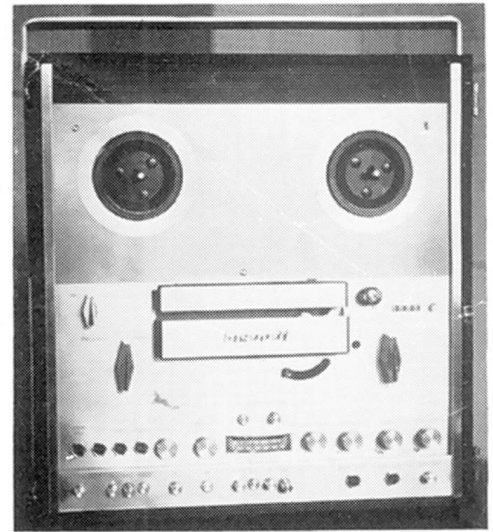
Latest model from Brenell Engineering is the Mark 6 Type M. It features pickup, ceramic and magnetic compensated inputs and a high quality replay amplifier with a 15 watt output. A/B switching facilities are provided to enable the recording to be compared with the original
