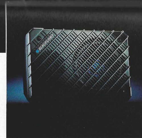
Blaupunkt BS 8720 B Broadband Loudspeaker, Surface Mount. Ref. No.: 7 606 898 000 Music Power Handling Capacity: 20 Watt Rated Power Handling Capacity: 8 Watt Frequency Response: 80–19,000 Hz Efficiency (1 Watt at 1 metre): 88 dB
