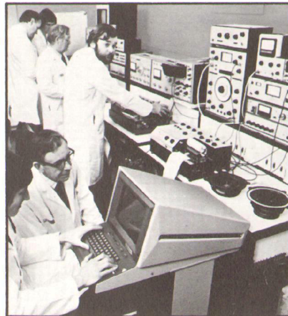
Computer-aided research in the B&W laboratory. Tektronix visual display unit in the foreground, B&K analogue equipment behind.
