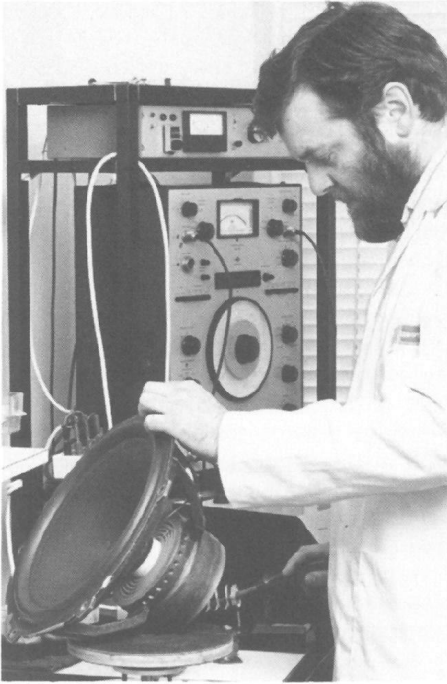
A prototype 801 low-frequency driver under construction.
