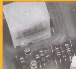
This illustration shows the APOC circuit within a crossover network.
