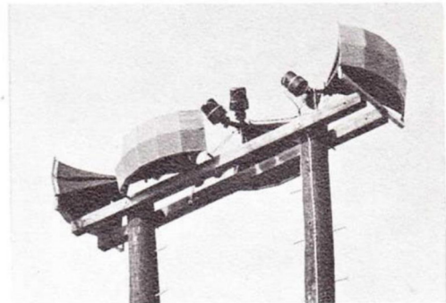
Multicellular Horns and Drivers mounted on tall buildings, poles, water towers, or specially built towers effectively cover a circle 2/3 of a mile across. Horns and equipment are impervious to dust and moisture.
