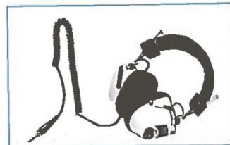
For monitoring, connect stereo headphones of 8 \Omega impedance to front panel Headphone Jack.
