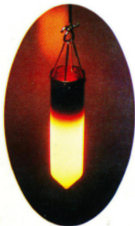
Platinum crucible during AKAI's ferrite melting process
