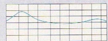
Headphone player frequency characteristics Other important features include: 60 Hz region: Boost to counteract leakage losses common with in-ear headphones. 10–20 kHz: Boost to counter deterioration in tape performance with outdoor use.
