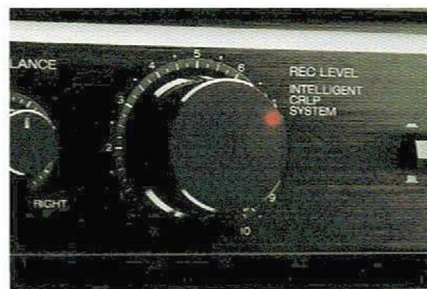
The CRLP switch on the front panel
