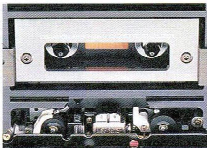
Transport mechanism with new ceramic composite tape guides
