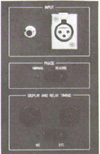
Input Terminals, Phase Inverting Switch and Synchronizing Signal Terminals at rear panel.
